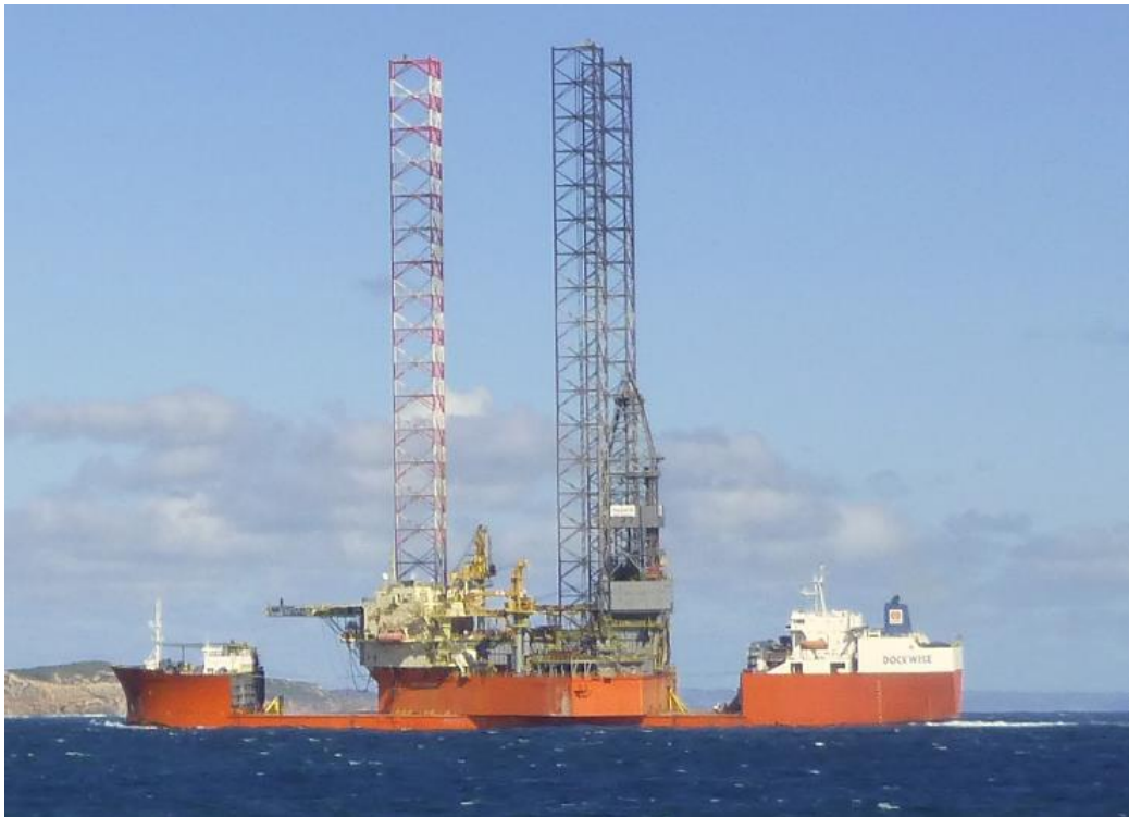
West Telesto drilling rig on transport ship
